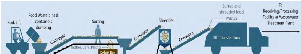
Figure 6: Marin Sanitation Service process schematic
